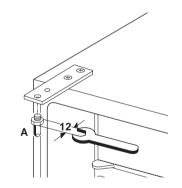
7. Unscrew the handle and refit it on the opposite side. Cover the holes left open with the plugs contained in the documentation pack.
